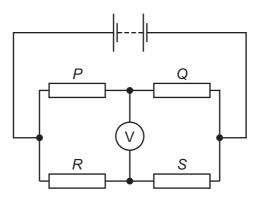
The voltmeter reading is zero.
